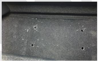
M6 Nutserts need to be fitted to the drilled holes. This can be done with a nutsert gun. Alternatively, the fitting kit comes with a small nutsert fitting device. Assemble the above components as shown. Use a small amount of lubricant between the bolt head and washer.
