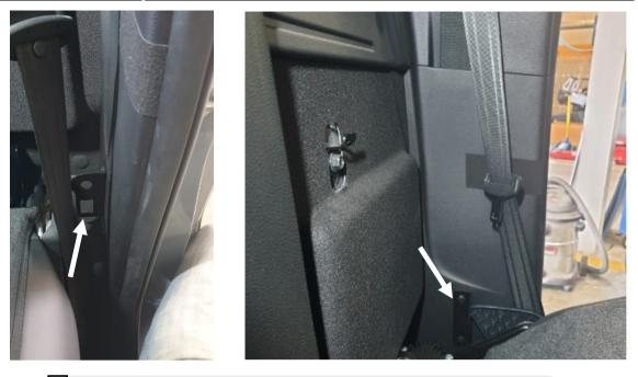
Reinstall the plastic trim. Bracket should be positioned as shown. Reinstall door jamb seal and scuff plate.
