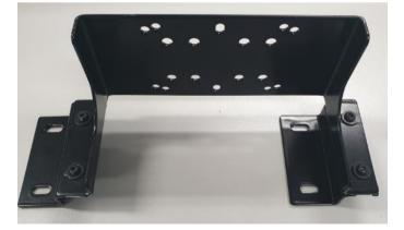
Loosely mount the feet to the compressor bracket using M6x20 bolts & M6 flat washers as shown. Please note the orientation of the feet.
