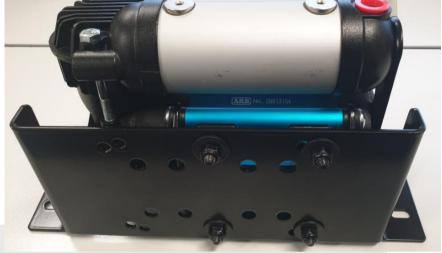
Mount the compressor bracket (with compressor bolted to it) onto the bracket feet using 4x M6x20 screws and M6 flat washers
