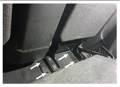
Sit the bracket assembly in desired position and mark the centre of the slotted holes with a permanent marker. (PX3 shown).
