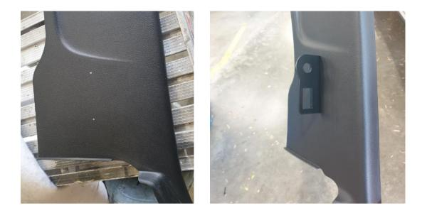
Drill out the mount holes to 7mm. Mount the bracket as shown using 2x M6x20 bolts, M6 flat washers & M6 flange nuts.
